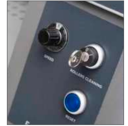
Electronic working speed adjustment by potentiometer
